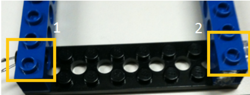
LEFT: IR LED(2) + Phototransistor(1) Used as a wide break beam
